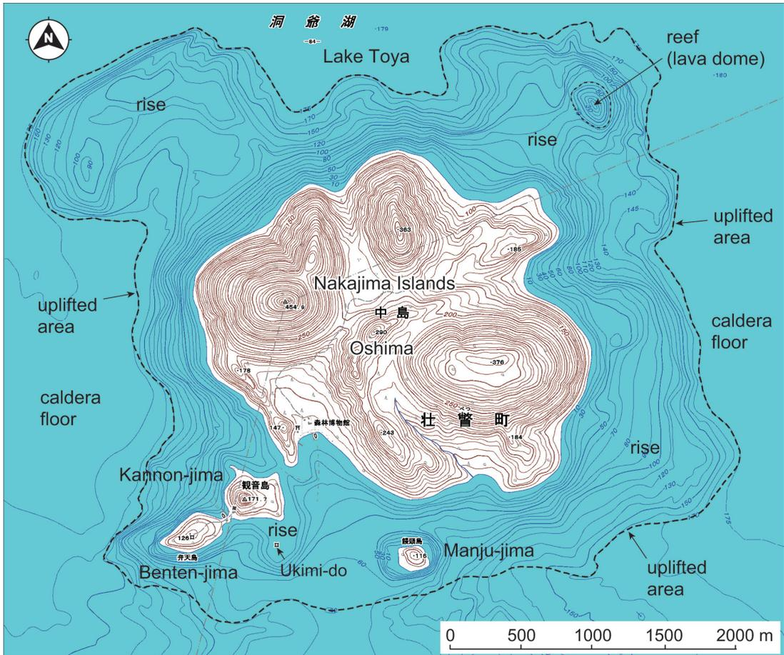
Fig. 3. Bathymetric map around the Nakajima Islands. The uplifted area is outlined by a dashed line. The location of a submerged lava dome (reef) is also shown. The base map was taken from the 1: 25,000 scale topographic map *Toya* issued by the Geospatial Information Authority of Japan (GSI). The topographic contour interval is 10 m.
