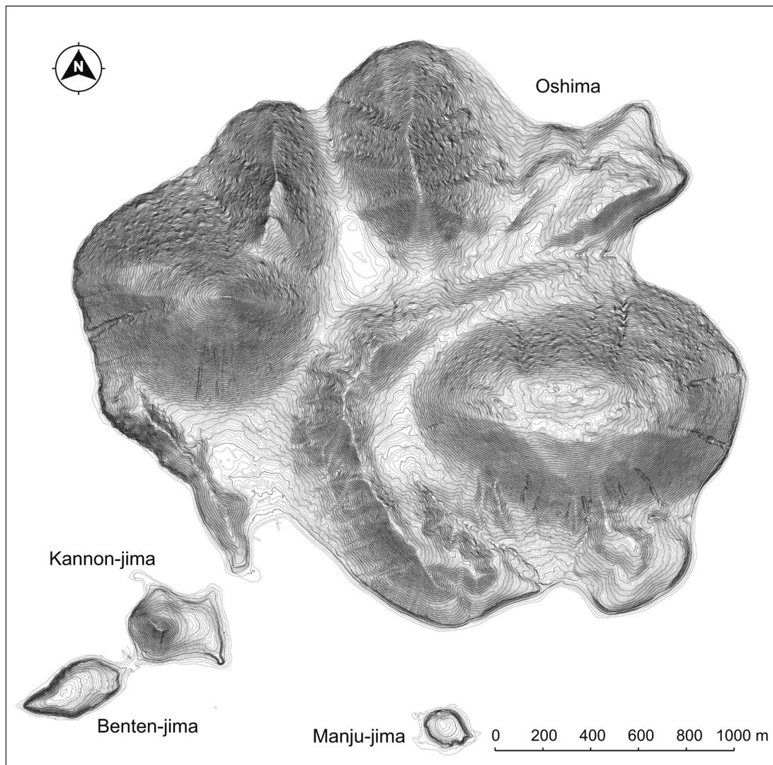
Fig. 6. Three-dimensional digital topographic map of the Nakajima Islands generated from the aerial laser-scanner mapping survey. The topographic contour interval is 2 m.
