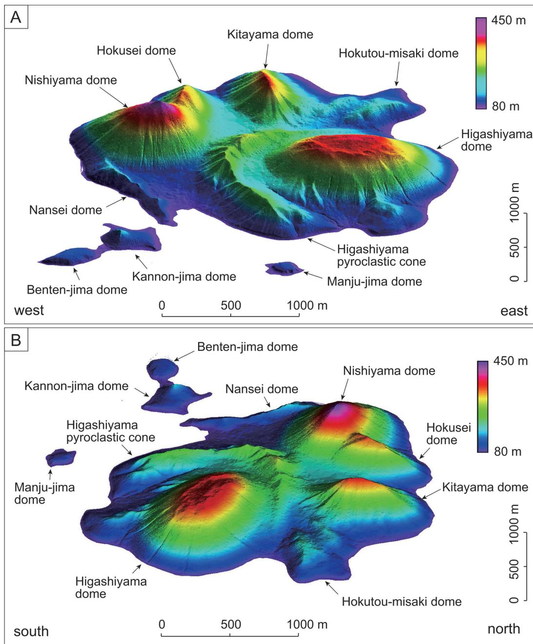
Fig. 8. Oblique three-dimensional digital images, produced by laser-scanner survey, of the Nakajima Islands viewed from the south (A) and east (B).
