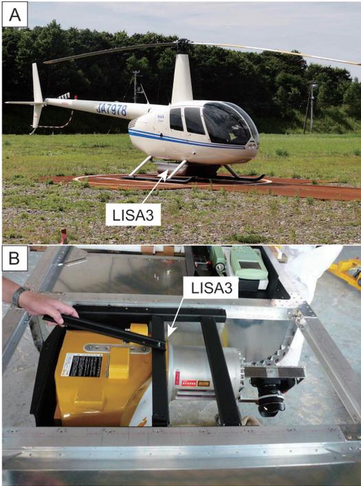
Fig. 4. (A) Photograph of the LISA3 instrument mounted on a manned helicopter. (B) Close-up photograph of the LISA3 instrument.
