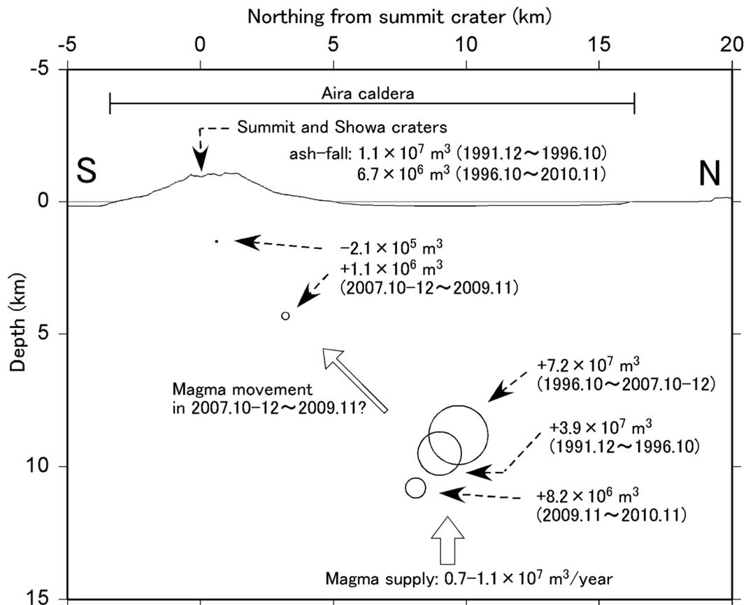
Fig. 6. Schematic illustration showing the locations of the calculated pressure sources projected onto North-South cross section crossing the summit crater of Sakurajima volcano (open circles) and inferred magma movement (see text for discussion). The results during the period of December 1991 - October 1996 (Eto *et al.*, 1997) are also plotted for comparison. The area of the each circle is drawn in proportion to the absolute deformation volume at the pressure source.
