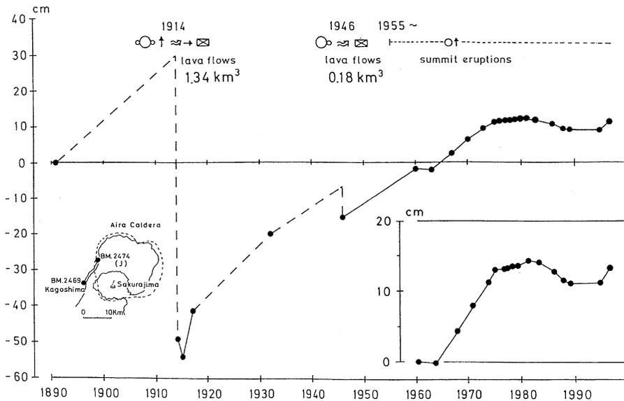
Fig. 5. Secular changes in the relative heights of BM.2474 referring to BM.2469 and the volcanic activity at Sakurajima (Eto *et al.*, 1997). The vertical displacement after 1960 is enlarged in a square in the lower-right corner. The dashed lines indicate an estimation based mainly on Sassa (1956). The volumes of the lava flows effused by the 1914 and 1946 eruptions are  $1.34 \text{ km}^3$  and  $0.18 \text{ km}^3$ , respectively.
