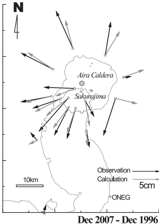
Fig. 6. Horizontal displacement vectors during the period from December 1996 to December 2007 (Iguchi *et al.*, 2008a). The solid and gray arrows show the observation and calculated vectors, respectively. The gray circle indicates the location of the Mogi pressure source. Station ONEG is used for reference.
