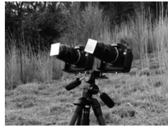
Fig. 1. (Top) Basic configuration of the SO 2 camera developed in the present study. (Bottom) SO 2 camera in field operation. Two CCDs are mounted alongside on a tripod.
