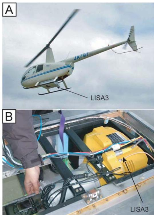
Fig. 2. (A) Photograph of the LISA3 instrument mounted on a manned helicopter. (B) Close-up photograph of the LISA3 instrument.
