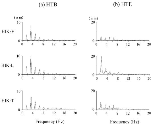
Fig. 4. Spectra of harmonic tremors. The spectra were obtained from 10s-seismograms at station HIK shown in Fig. 3. (a) Spectra of HTB from 16: 12: 55. (b) Spectra of HTE from 11: 21: 00.
