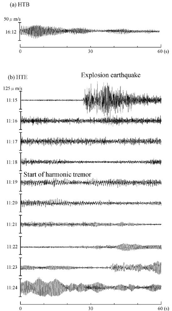
Fig. 2. Seismograms of harmonic tremors. The seismograms are observed by a vertical component of seismometer at station HIK. (a) HTB occurred on July 20, 1990. (b) Explosion earthquake occurred at 11: 15 on October 11, 2002 and HTE started at 11: 19.
