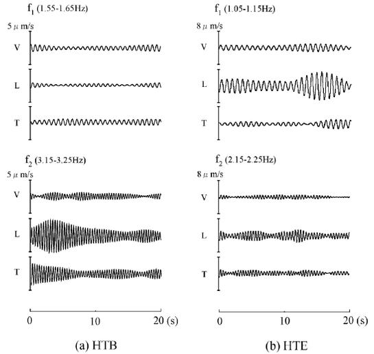
Fig. 5. Examples of waveform band-pass filtered at  $f_1$  and  $f_2$  with band width of  $\pm 0.05$  Hz. Seismograms are observed at station HIK. (a) HTB from 16: 12: 55 to 16: 13: 15 on July 20, 1990. (b) HTE from 11: 19: 00 to 11: 19: 20 on October 11, 2002.
